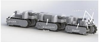
Sensors located inside the robot
